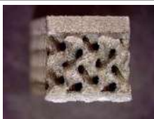
Figure 7.11: Gyroid structure for thermal management
