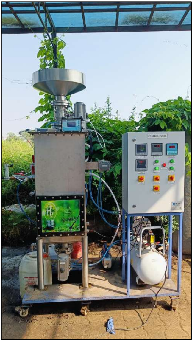
Green Hydrogen Production using metal scrap and sea water
