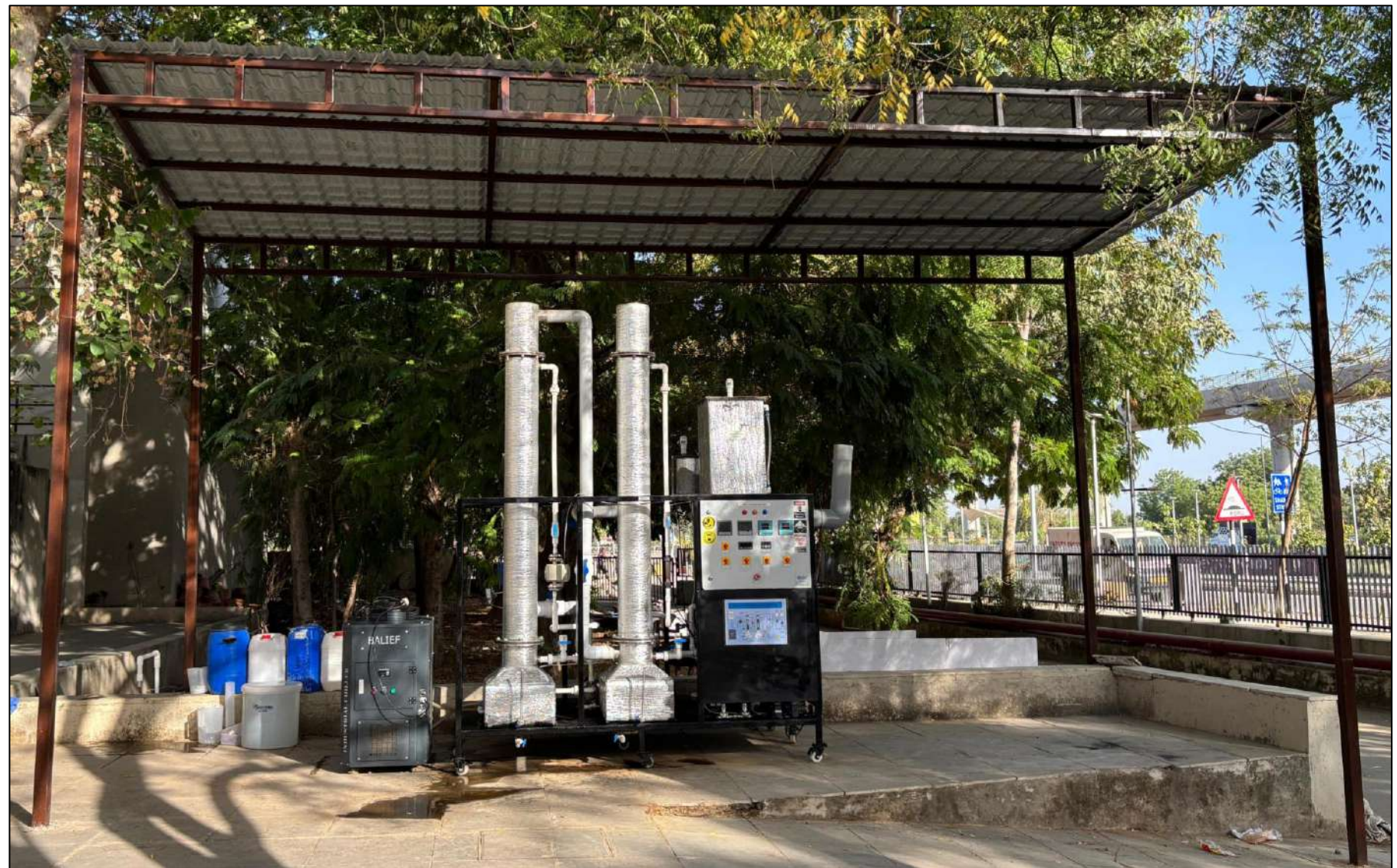
Direct Air CO 2 Capture Plant – Enable to capture CO 2 from various locations using different potential solvents
