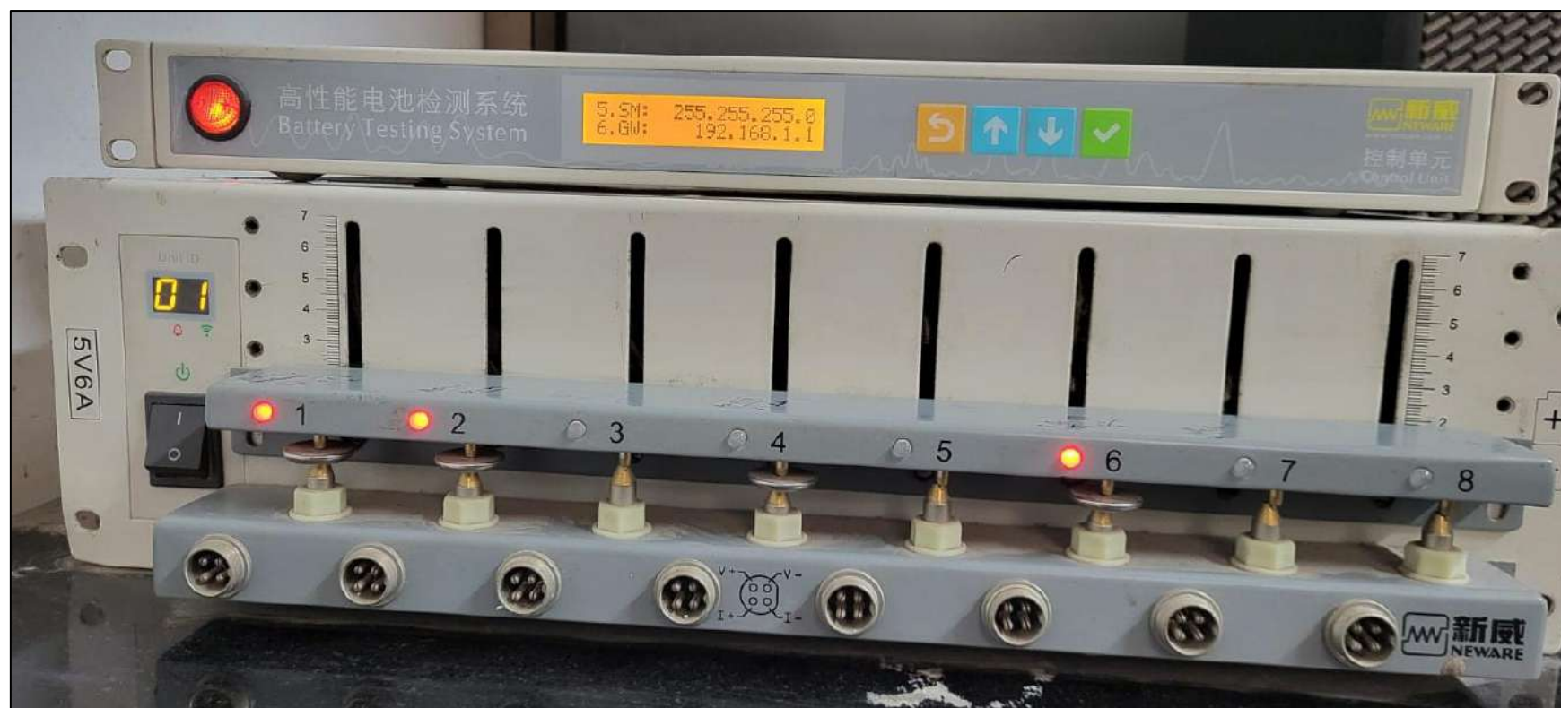
Battery Tester – Evaluates battery performance, health, and efficiency
