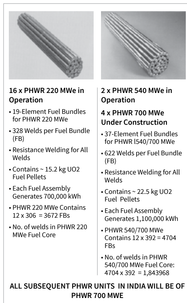
FIGURE 5. PHWR 220 and PHWR 540/700 Fuel Assemblies Manufactured at NFC routinely
