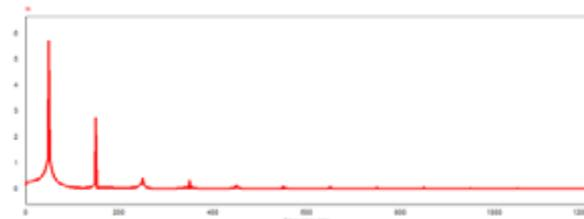
FIGURE 6: FFT Analysis of Supply current (Is)
