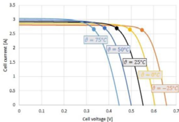
Figure 2: Solar PV performance at various operating temperatures
