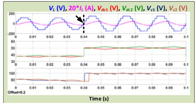
Figure 5: Results under sudden increase in input voltage
