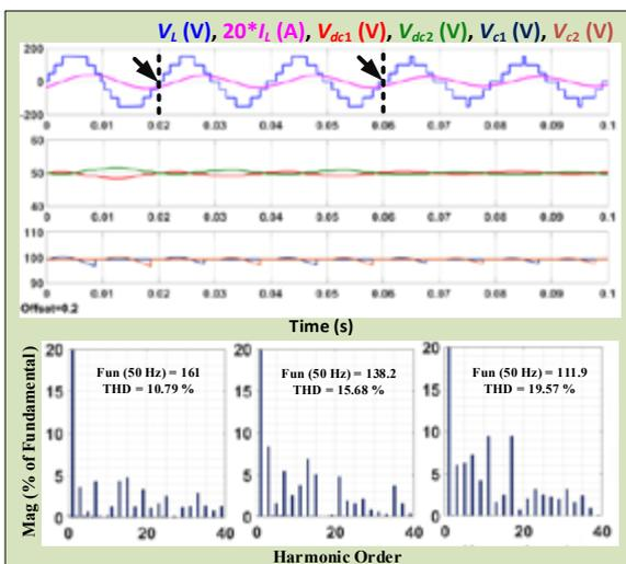
Figure 4: Results under a change in modulation index
